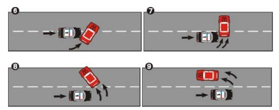
Once the rear of the suspect vehicle has been moved past 25-30 degrees from the original path of travel, the rotation is irreversible. The suspect vehicle will continue to rotate regardless of any action taken by its driver, including counter steering, braking, or accelerating.
